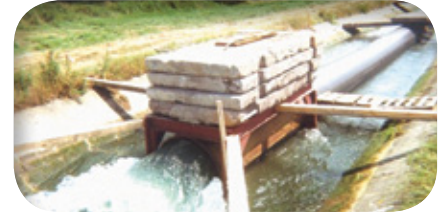
Figure 2: Hydraulic test of HDPE pipes in Poland (Technical University Swietokrzyska).
