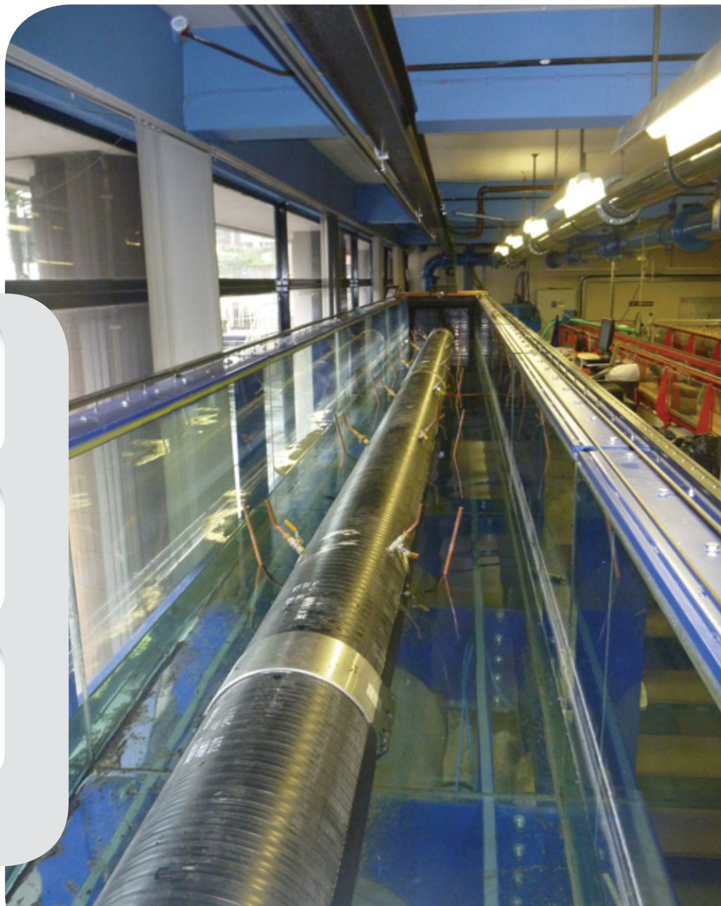
Figure 2: Hydraulic test of HDPE pipes in Poland (Technical University Swietokrzyska).
